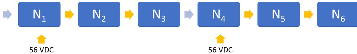
Figure 4 Six units connected in series with power being supplied via two 56VDC supplies. This configuration can support simultaneous operation of all units.
