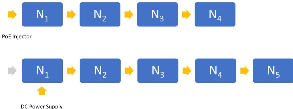
Figure 5 Two Configurations for linear networks where a single unit is powered for RFID operation at any given time. The upper diagram shows N1 powered by the SensThys injector, with the lower diagram shows the string of units powered by the SensThys DC supply.
