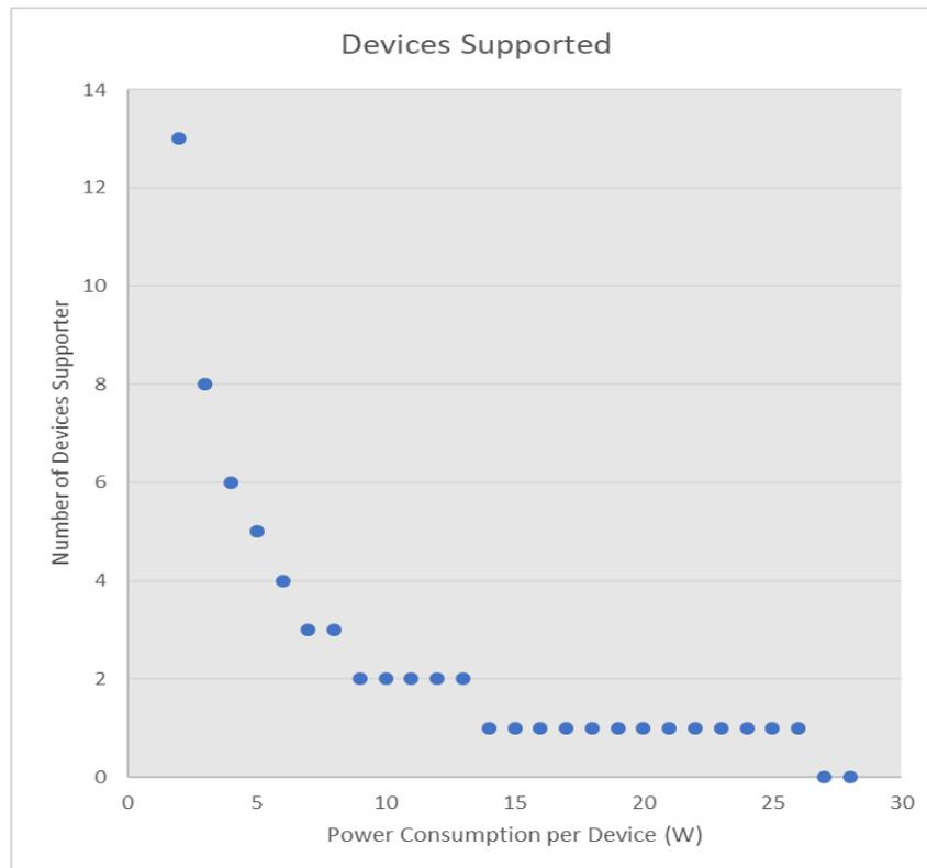
Figure 2 The number of devices supported by a single PoE+ supply. As the power consumed per device decreases, the number of devices supported increases.
