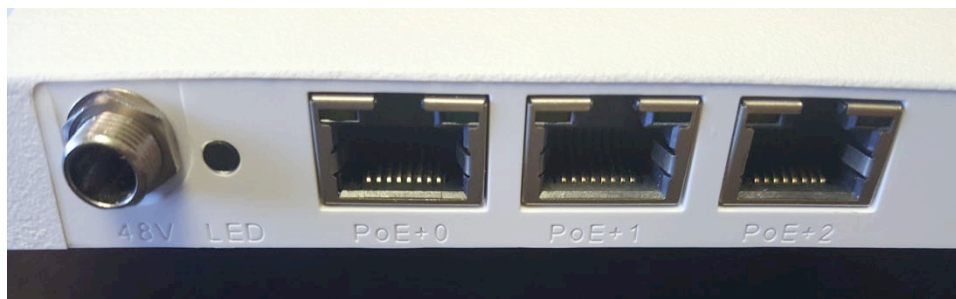
Figure 5: Detail of labels for the 56V input, the Status LED and the Ethernet ports on SensArray Pro unit.
