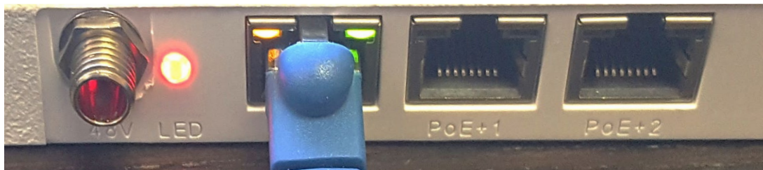
Figure 11: The SensArray in the process of booting. The LED flashes red.
