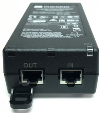
Figure 1: Metallic trim on RJ-45 ports on shielded RJ-45 connector on PoE+ injector P/N POE29U-1AT (left), 56VDC power supply (right)
