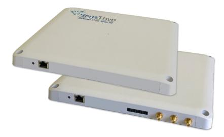
The SensArray® One Series combines one of the strongest, fastest UHF passive RFID readers with an integrated 8.5dBic antenna in a svelte, attractive 10" x 10" form-factor. The reader operates at a full industry maximum of +33dBm via the 90W Class 8 PoE input, so no separate DC power input is required.
