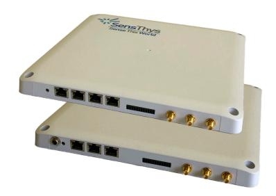
The new SensArray Pro and Enterprise readers combine one of the strongest, fastest UHF passive RFID readers with an integrated 8.5dBic antenna in a svelte, attractive 10" x 10" form-factor. The SensArray Enterprise operates at a full industry maximum of +33dBm via the 90W Class 8 PoE input, so no separate DC power input is required. The SensArray-Pro operates at 30dBm with Class 4 30W PoE input.
