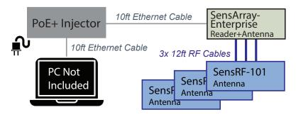
This kit includes the SensArray-*Enterprise* which is a novel RAIN RFID **reader** that also contains an 8.5dBic **antenna**, network **switch** and **power distribution** system. Combined these massively reduce infrastructure and installation costs. All of these elements are consolidated into a svelte, attractive 10" x 10" form-factor. The SensArray *Enterprise* operates at a full industry maximum of +33dBm via the **90W Class 8 PoE** input, so no separate DC power input is required.
