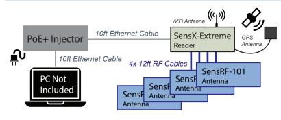
This kit includes the new SensX EXTREME rugged reader which is enclosed in the industry's highest rated IP67 industrial and weather-tight chassis. Operators can now install RFID reader networks in places where traditional readers have previously not been suited, inside or out. No NEMA box required!
