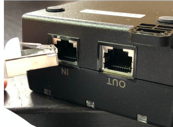
Figure 3 - PoE Injector with metal shield socket and Ethernet cable with metal shield surround (see Step 3)
