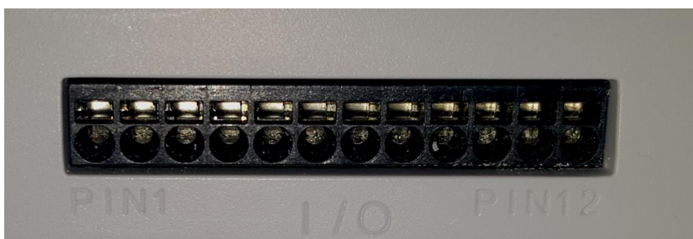
Figure 6 The GPIO port, labeled "I/O"
