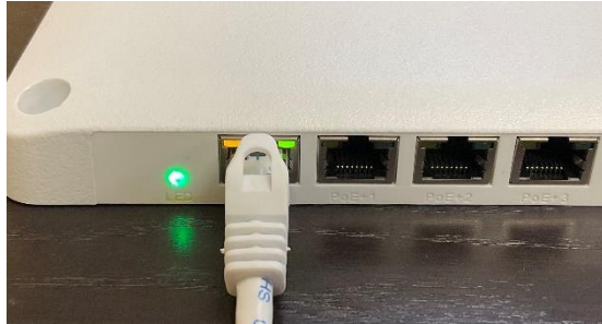
Figure 5: Detail of labels for the Status LED and the Ethernet ports on an Enterprise unit.
