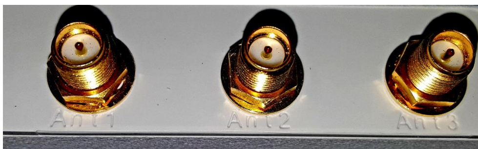
Figure 8: The three reverse-polarity SMA connectors for external antennas.
