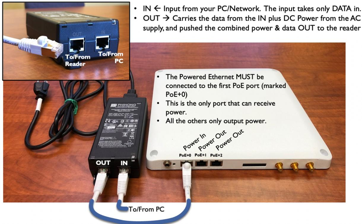
After powering your SensThys reader and launching the RFID Console, the POE switch or injector commences the hand-shaking procedure with the unit, culminating in the Enterprise or Core being fully powered. Next, the CPU boots up, setting up its power architecture and becoming ready for operation.
