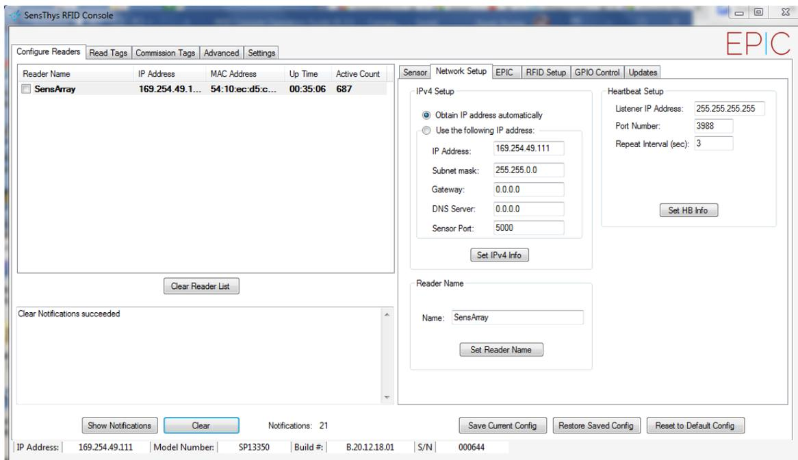
Figure 6: The Network Setup tab in the Console
