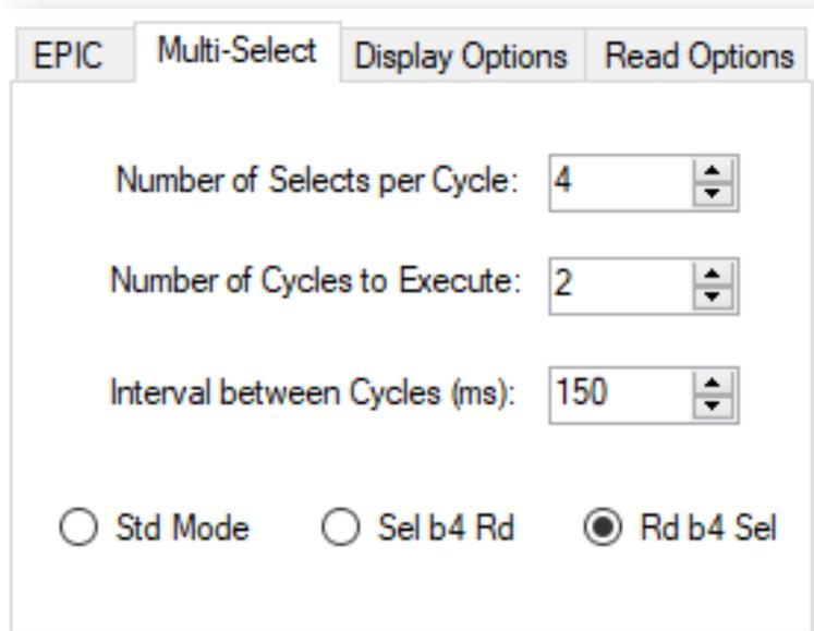
This combination of settings will allow you to see all the tags that are visible to the reader, in Sensitive mode, but will generally only read each tag once, thus minimizing the tag read traffic and providing quite stable Console operation.
