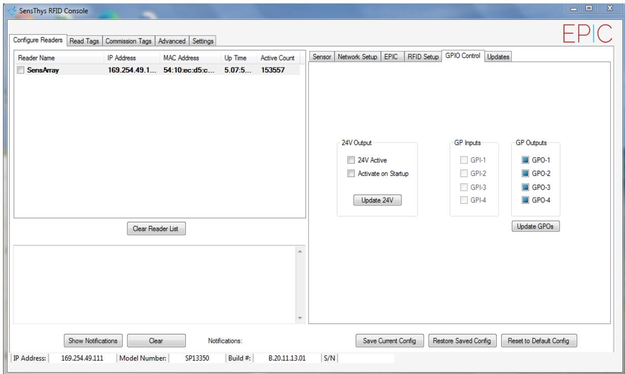
Figure 11: The GPIO Control tab in the Console
