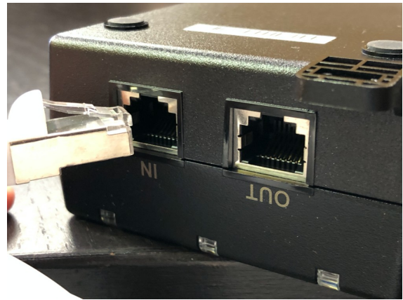
Figure 24 - PoE Injector with metal shield socket and Ethernet cable with metal shield surround (see Step 3)
