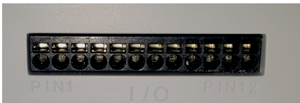
Figure 1 The GPIO port, labeled "I/O"
