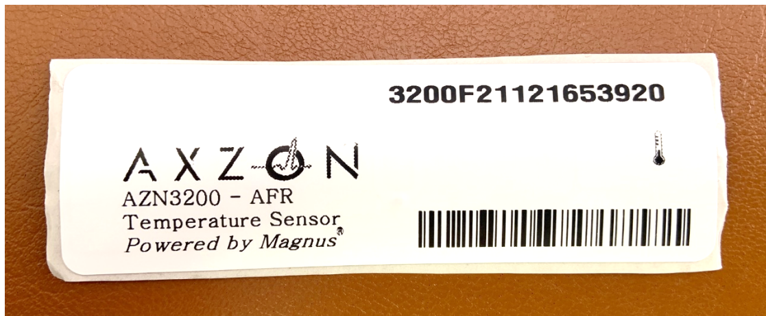
Figure 5 - The sensor with a front label. The label can include information stored on the tag and information helpful in the customer environment.
