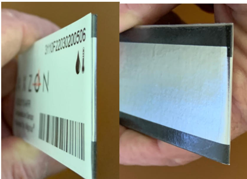
Figure 13 - The other end, showing the bottom metal in contact with the top portion. This is the “shorted end”. Shown from the top (left) and bottom (right).
