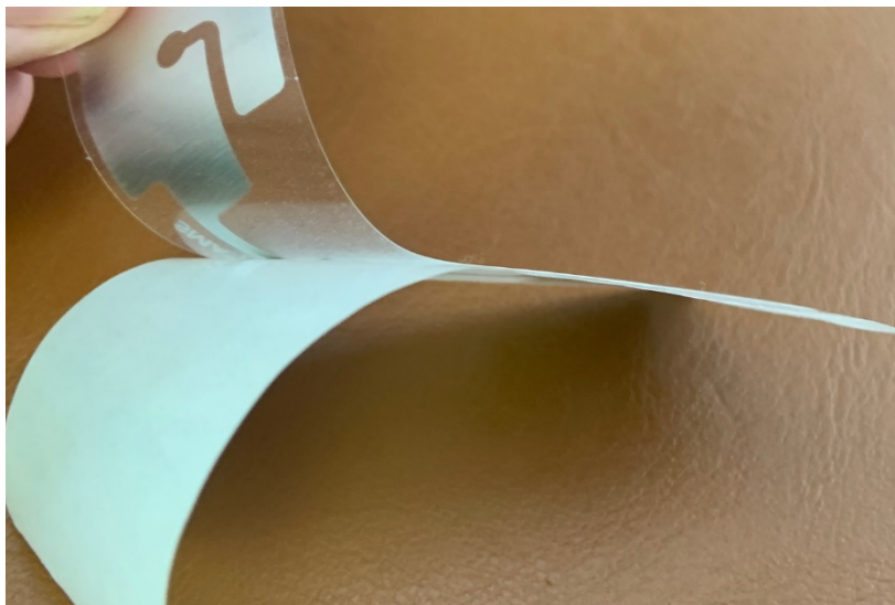
Figure 4 - The inlay, with an adhesive on the back being removed from the backing material.
