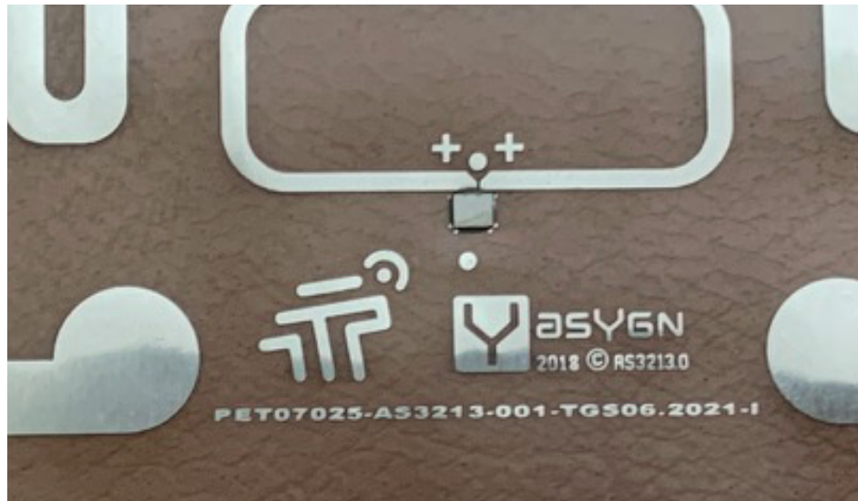
Figure 2 - The sensor die. For scale, the word “ASYGN” is 7 mm across.
