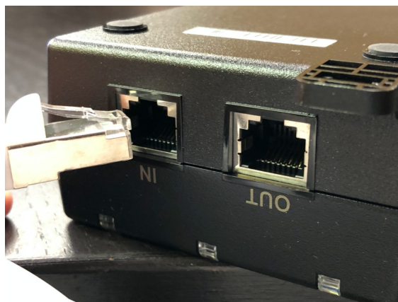
Figure 24 - PoE Injector with metal shield socket and Ethernet cable with metal shield surround (see Step 3)
