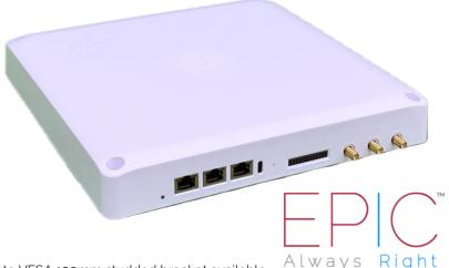
The reader is supplied as a flat/through-hole mount with a separate VESA 100mm studded bracket available (allowing mounting to a standard VESA mount).
